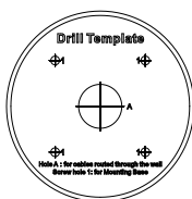
Figure 2-20 Drill Template of the Junction Box
